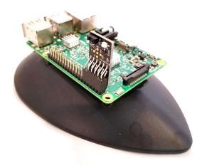
The IR components should face outward from the Pi, and ideally toward your couch. PiRCy sits at the very end of the 40-pin GPIO header.
