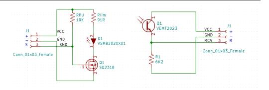
For the sender side, the Rlim of 910hms corresponds to roughly 40mA from a 5V supply. A small MOSFET is placed to enable the IR LED from a standard GPIO rather than sourcing it directly.
