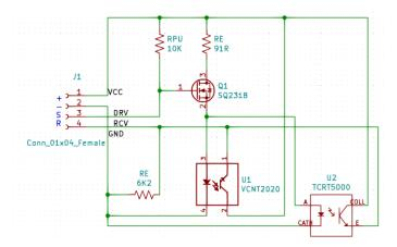
The RE (emitter resistance) of 910hms corresponds to roughly 40mA from a 5V supply. A small MOSFET is placed to enable the IR LED from a standard GPIO rather than sourcing it directly. Only ONE sensor should be installed, as they share outputs.
